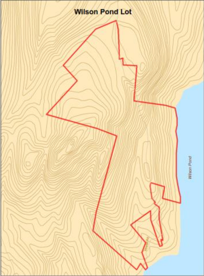
215 216 217 Figure 2. Contours (10 ft. interval) of the Wilson Pond Lot 218 showing greater than 20% slope.
